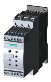
SIRIUS SOFT STARTER, S0, 32A, 15KW/400V, 40 DEGR., AC 200-480V, AC/DC 24V, SCREW TERMINALS
